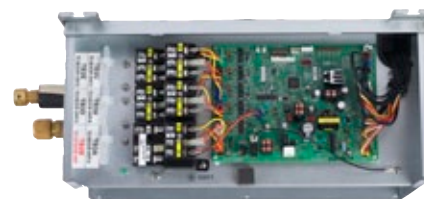
PAC-AKA51BC Electrical Board
